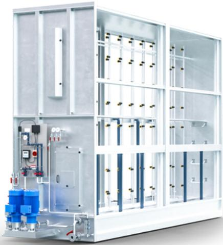
The circulating water spray humidifier, also called an air washer, is a classic among humidification systems. The volume of water atomised within the air flow is several times greater than the water flow required for humidification. The water that is not evaporated is captured in a tank and recirculated to the nozzles.
